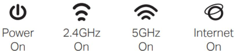
Note: If the 2.4GHz LED and 5GHz LED are off, press and hold the WPS/Wi-Fi button on the back for more than 2 seconds, then release the button. Both the LEDs should turn solid on.
