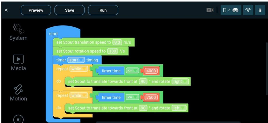
This graphical program generates Python codes and runs on Scout's ROS system. The Scout Scratch modules are divided into several categories, System, Media, Motion Control, Ai functions, Logic, Math, Loops, Lists, and Variables. Among them, Logic, Math, Loops, Lists, and Variables are standard modules by Blockly.
